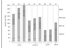
Figure 4 Carbon footprint of different PV systems indicating the solar module carbon emission dominance. Balance of system (BOS) includes typically includes inverters, mounting structures, cable and connectors<sup>10</sup>
